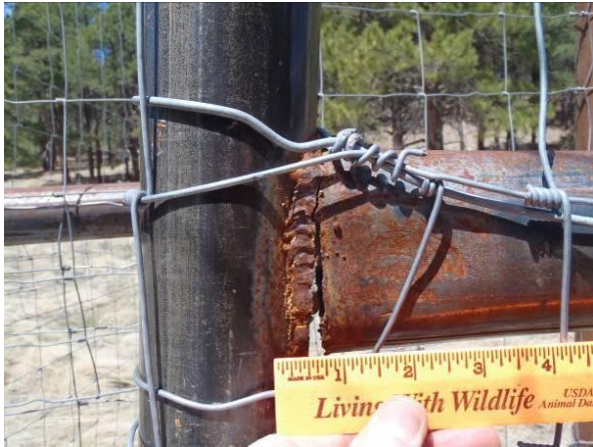
Figures 31 and 32. Cracked welds, April 2011.
