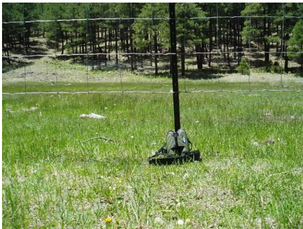
Figure 4. Example of height from ground to bottom wire
